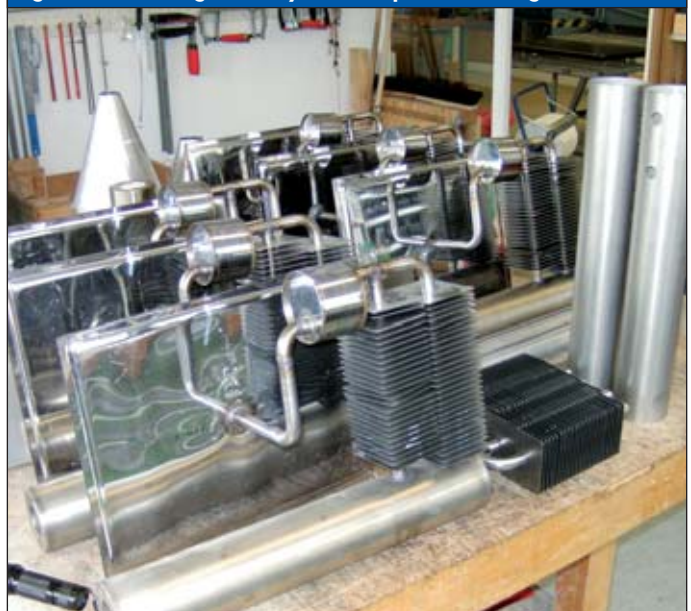
Fig. 5: Zeolite refrigeration systems for practical testing
